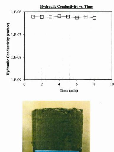
Note: A B-value of 0.97 was achieved for the undisturbed specimen. Permeation measurements were made with a mercury Utube. The effective confining pressure was 5 psi per test request.
