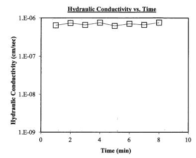
Note: A B-value of 0.95 was achieved for the undisturbed specimen. Permeation measurements were made with a mercury Utube. The effective confining pressure was 5 psi per test request.
