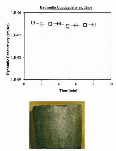
Note: A B-value of 0.97 was achieved for the undisturbed specimen. Permeation measurements were made with a mercury Utube. The effective confining pressure was 5 psi per test request.
