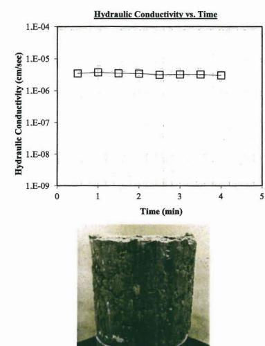
Note: A B-value of 0.96 was achieved for the undisturbed specimen. Permeation measurements were made with a mercury Utube. The effective confining pressure was 5 psi per test request.
