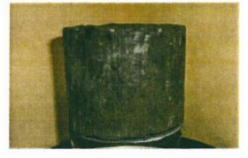
Note: A B-value of 0.95 was achieved for the undisturbed specimen. Permeation measurements were made with a mercury Utube. The effective confining pressure was 5 psi per test request.
